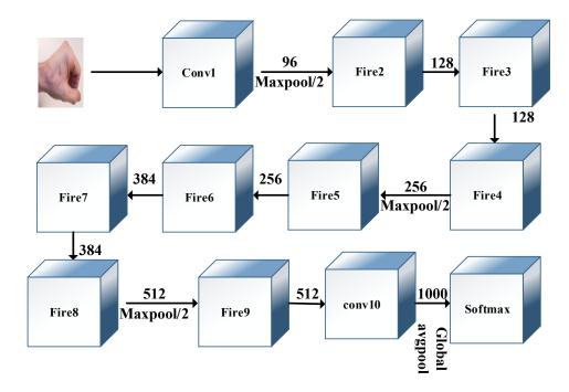
Figure 2. SqueezeNet Architecture [30]
