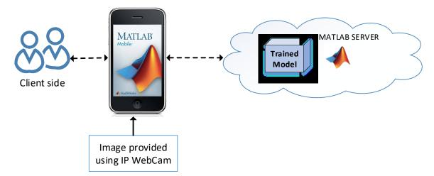
Figure 4. Client-server architecture-based framework for the i-Rash mobile application
